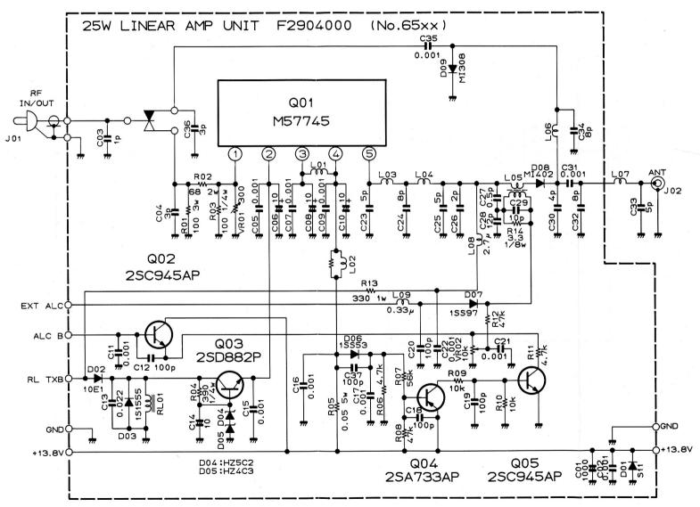
RESISTOR VALUES ARE IN  $\Omega.1/6w$ : CAPACITOR VALUES ARE IN  $\mu F.50wv$ : INDUCTOR VALUES ARE IN HENRIES: UNLESS OTHERWISE NOTED.
